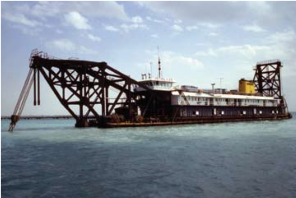
Cutterhead dredge at Jiddah, February 1978
